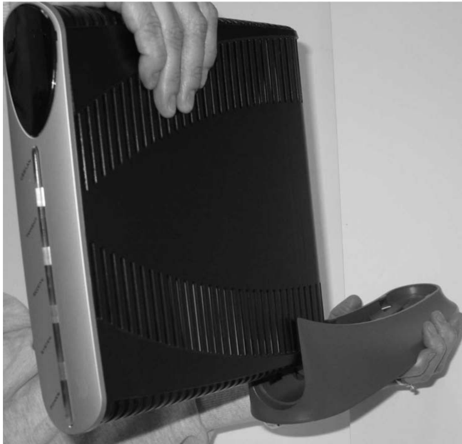
Figure 25: Orienting pedestal base and DW6000
