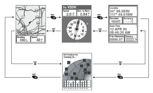
*Tip:* The **ESC** button will also set through the navigation screens, just like the **NAV** button but in the reverse order.
