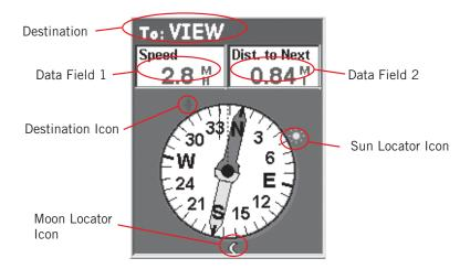
The top of the screen (the header bar) displays the name of the destination if you have an active route. Without an active route, the destination name is blank.
