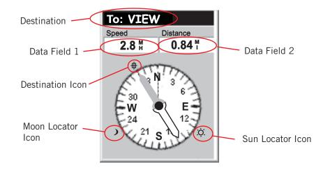
The top of the screen (the header bar) displays the name of the destination if you have an active route. Without an active route, the destination name is blank.
