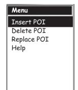
*Deleting:* Use the **Arrow** joystick to highlight the POI you want to delete from the route. Press **MENU**, highlight **Delete POI**, and press **ENTER**.
