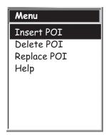
*Deleting:* Use the **Arrow** joystick to highlight the POI you want to delete from the route. Press **MENU**, highlight **Delete POI** and press **ENTER**.
