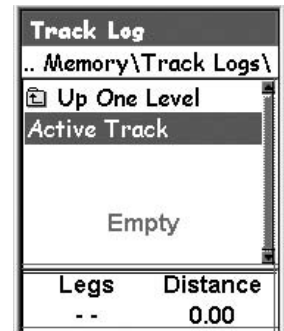
Track Log List with information at the bottom for the number of legs and the distance of the track log highlighted
