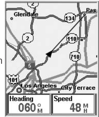
Map screen with a GOTO route active. Notice the line on the screen that graphically displays the route.
