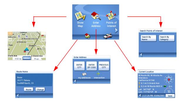
**Show Map:** Displays the map with your current position (if computing a position from the GPS signals) indicated by the blue triangle. See the Map Screen chapter for details.
