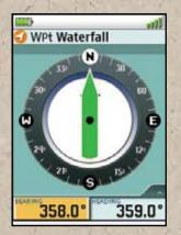
The Triton 1500's compass screen provides precise heading and bearing information.
