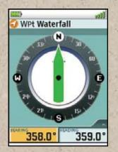
The Triton 300's compass screen provides precise heading and bearing information.
