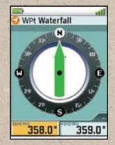
The Triton 400's compass screen provides precise heading and bearing information.
